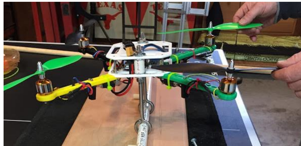
Test stand for PID and motor trim tuning.
