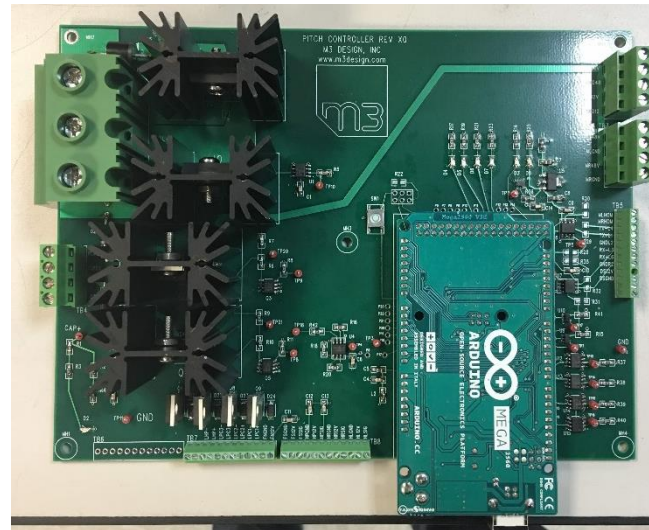
Surface-mount soldered 50+ circuit elements to PCB for ball-toss machine and programmed Arduino charge/discharge control.
